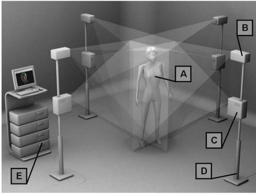
**Fig. 2** A visualization of a patient (a) being measured in the system. Each measurement module consists of (b) a CCD camera and (c) a DLP projector (d) fixed to a stand and (e) is controlled by a computer.
