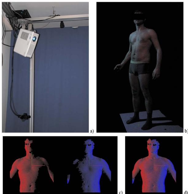
**Fig. 3** The measurement setup in the laboratory at the Institute of Micromechanics and Photonics: (a) a directional measurement module fixed to a stand, (b) a healthy individual lighted with a fringe pattern from the module in (a), (c) the two front (+45 and -45 deg) out of four directional point clouds representing the patient's upper body surface, and (d) the front clouds merged automatically based on the global coordinate set calibration.
